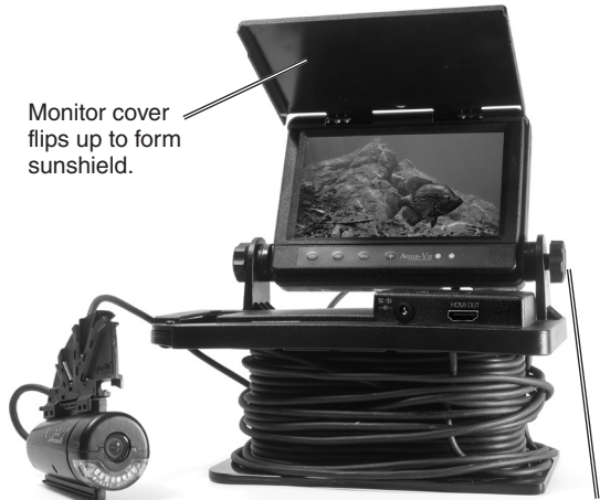
Rotate the circular knobs to adjust the angle of the monitor
