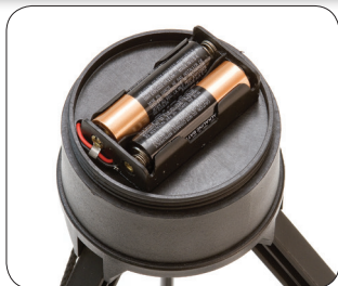
BATTERY PLACEMENT UNDER TOP CAP
